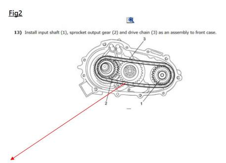
Chain repair kit - this is the area where the noise is experienced due to the vibration of the chain when vehicle takes off in first gear at around 2000rpm.
