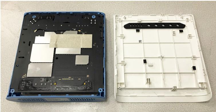
6. Remove the 4 screws from the mainboard.
